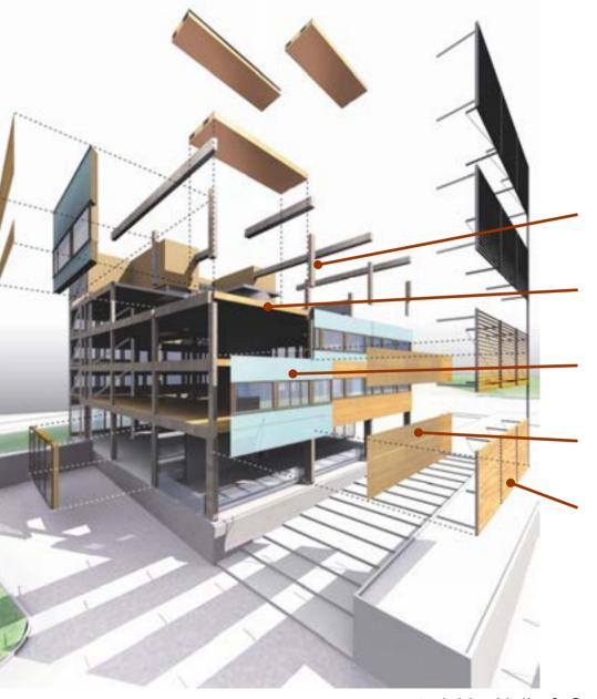
PREFABRICATION lessens essentially the work carried out on the building site.
